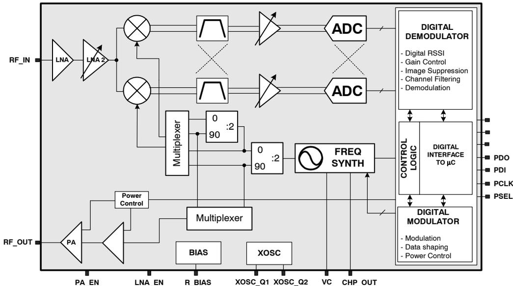
Figure 2. **CC1020** simplified block diagram
