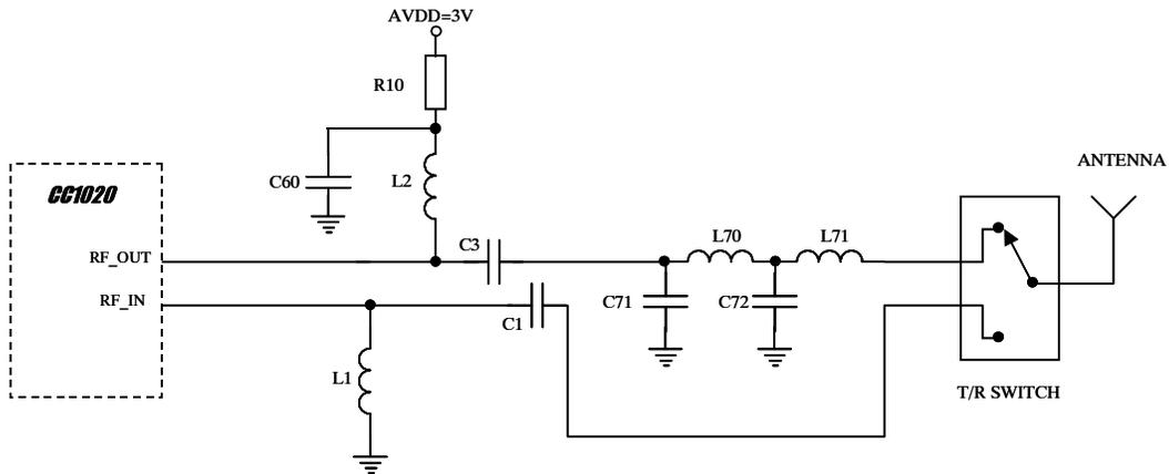
Figure 25. Input/output matching network
