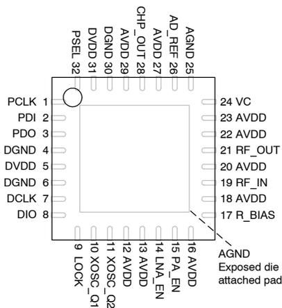
Figure 1. **CC1020** package (top view)
