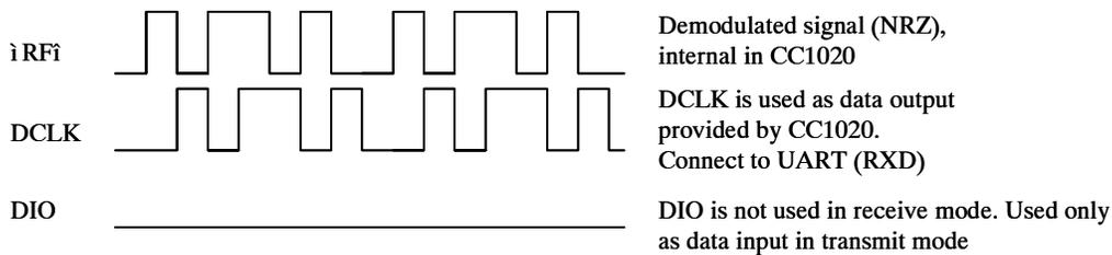
Figure 11. Transparent Asynchronous UART mode ( $SEP\_DI\_DO = 1$ )
