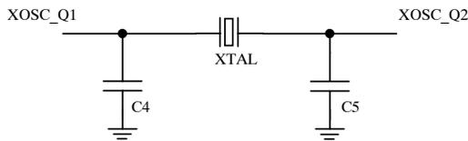
**Figure 33. Crystal oscillator circuit**
