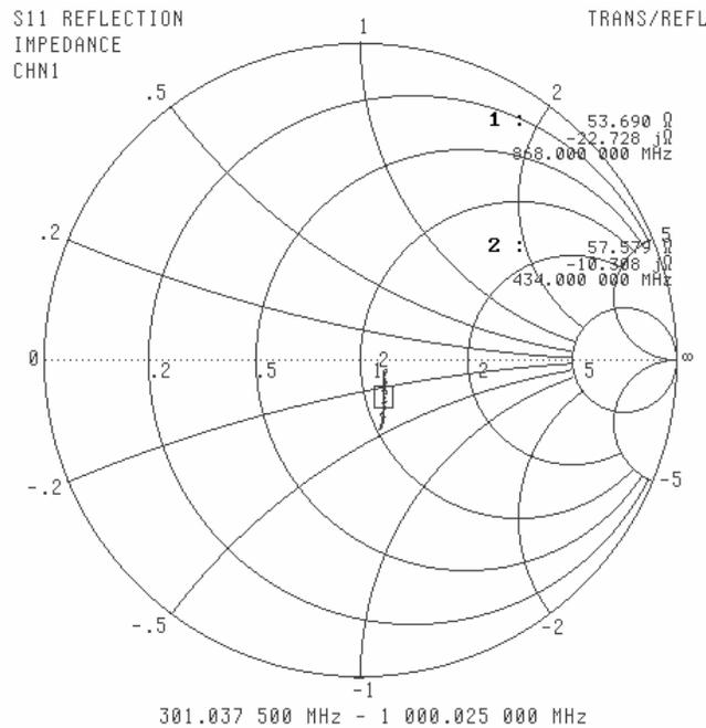
Figure 26. Typical LNA input impedance, 200  $\mu$  1000 MHz
