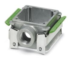
DUPLICON, aluminum stackable housing for DUPLICON contact inserts, type B6, IP67 protection, with two locking latches, gasket and an M20 cable screw connection thread (without cable screw connection)
