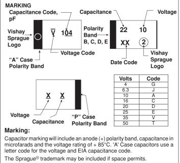
Units rated at 6.3 V shall be marked 6 V.
