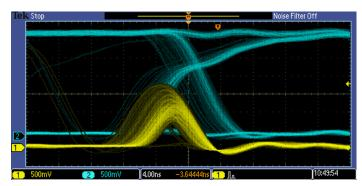
Digital phosphor technology enables a 5,000 wfm/s waveform capture rate and real-time intensity grading on the MSO/DPO2000B Series.
