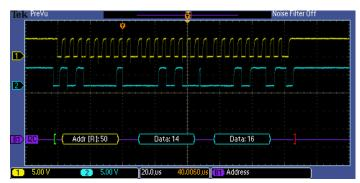
Triggering on a specific data packet going across an I<sup>2</sup>C bus. The yellow waveform is clock and the blue waveform is data. A bus waveform provides decoded packet content including Start, Address, Read/Write, Data, and Stop.
