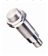
The GS1001-1002 series gear tooth sensors are Hall Effect devices designed for use in applications where ferrous edge detection or near zero speed sensing (without power up recognition) is needed. Current sinking output requires the use of a pull up resistor. Circuit protected with adjustable stainless steel housing
