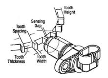
For best results, we recommend targets made from low carbon cold rolled steel. Other factors that influence sensor performance include geartooth height and width, space between teeth, shape of the teeth and thickness of the target. As a general guideline, consider a target with the following minimum parameters:
