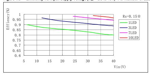
Figure 1.4 Efficiency vs. Input Supply Voltage  $(V_{IN} = 8.5 \text{ to } 40\text{V})^{\ddagger}$  Per Number of LEDs (Rs=0.30 $\Omega$ , L1=47 $\mu$ H)
