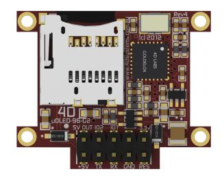
This microOLED module can be programmed in its native 4DGL language (similar to C), using the Workshop 4 IDE Software tool suite. It can also be configured very easily as a serial slave device, for use with your favourite host controller. Freedom is at your fingertips with the intelligent  $\mu$ OLED-96-G2 display module.
