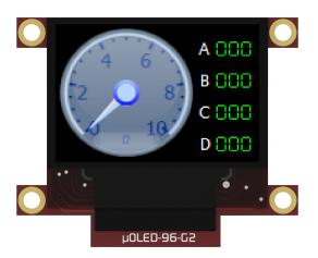
Embedded at the heart of the design is the **GOLDELOX** processor, which is driven by a highly optimised virtual core engine called **EVE** (Extensible Virtual Engine).
