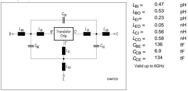
The SOT343 package has two emitter leads. To avoid high complexity to the package equivalent circuit both leads are combined in one electrical connection
