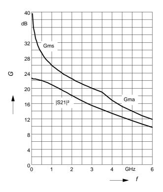
**Power gain**  $G_{ma}$ ,  $G_{ms} = f (V_{CE})$  $I_{C} = 5 \text{ mA}$
