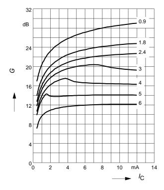
**Power gain**  $G_{ma}$ ,  $G_{ms}$ ,  $|S_{21}|^2 = f(t)$  $V_{CE} = 2 \text{ V}$ ,  $I_C = 5 \text{ mA}$
