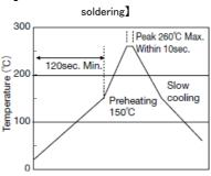
①Wave soldering must not be applied to capacitors designated as for reflow soldering only.
