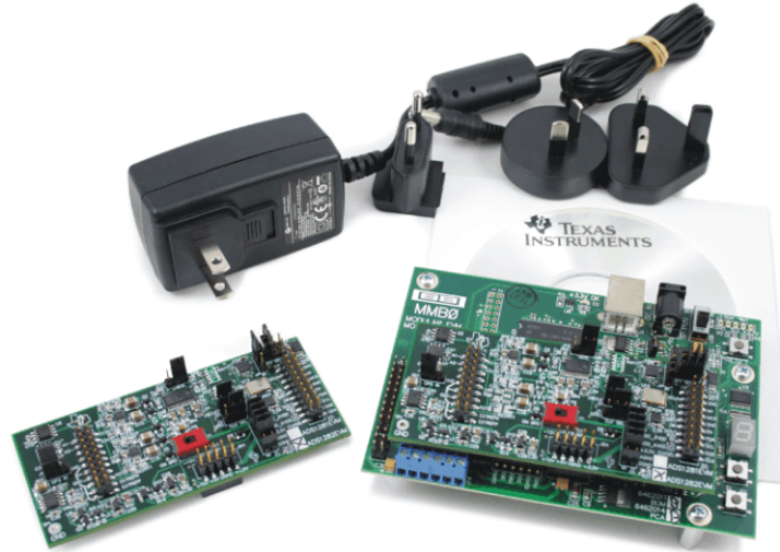
ADS1282EVM (Left) and ADS1282EVM-PDK (Right)
