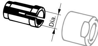
Sleeve «B» for connectors with PEEK or PBT insulators
