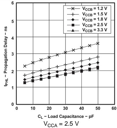
Figure 8. Typical Propagation Delay t<sub>PHL</sub> (A to B) vs Load Capacitance
