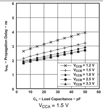
Figure 4. Typical Propagation Delay t<sub>PHL</sub> (A to B) vs Load Capacitance
