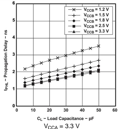
Figure 10. Typical Propagation Delay t<sub>PHL</sub> (A to B) vs Load Capacitance
