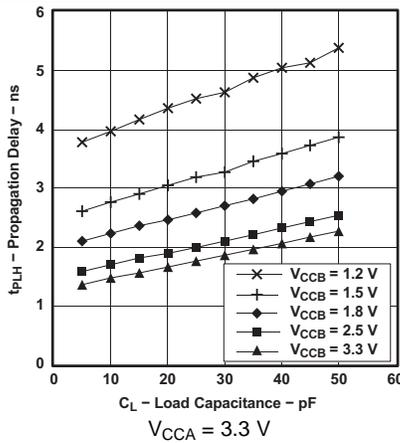
Figure 9. Typical Propagation Delay t<sub>PLH</sub> (A to B) vs Load Capacitance
