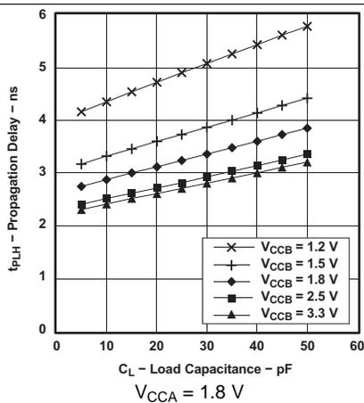
Figure 5. Typical Propagation Delay t<sub>PLH</sub> (A to B) vs Load Capacitance
