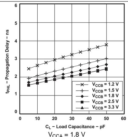
Figure 6. Typical Propagation Delay t<sub>PHL</sub> (A to B) vs Load Capacitance
