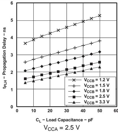
Figure 7. Typical Propagation Delay t<sub>PLH</sub> (A to B) vs Load Capacitance
