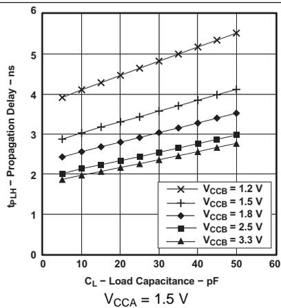
Figure 3. Typical Propagation Delay t<sub>PLH</sub> (A to B) vs Load Capacitance
