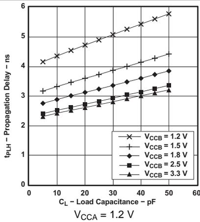
Figure 1. Typical Propagation Delay t<sub>PLH</sub> (A to B) vs Load Capacitance
