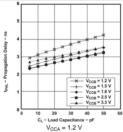
Figure 2. Typical Propagation Delay t<sub>PHL</sub> (A to B) vs Load Capacitance
