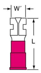
This female disconnect accepts a wire range of 22-18 AWG, a stud size of .187 and has a case quantity of 10 bags.
