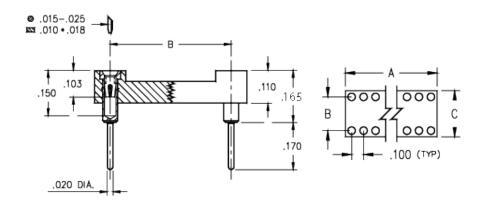
**Description:** DIP Socket Solder Tail Long Solder Tail (0.170 Tail) Open Frame Through Hole Plating Code: 93 Shell Plating:
