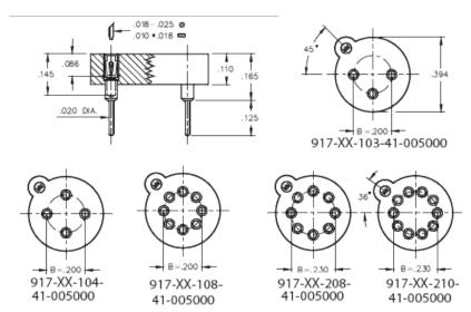
**Description:** Transistor TO Socket Through-Hole Mount Accepts .015"- .025" (0,38 - 0,635 mm) dia leads Through Hole Plating Code: 43 Shell Plating:
