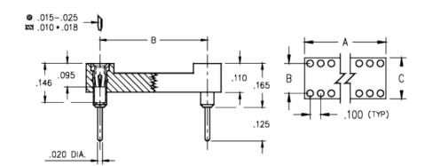
**Description:** DIP Socket Solder Tail Standard Solder Tail (0.125 Tail) Open Frame Through Hole Plating Code: 43 Shell Plating: 200 μ" Tin (matte finish) over 100 µ" Nickel
