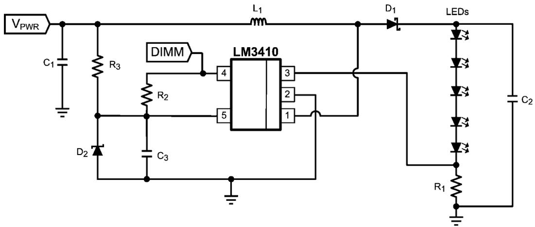
LM3410X (1.6MHz):  $V_{PWR} = 9V$  to  $14V$ , ( $V_{OUT} \approx 16.5V$ )  $I_{LED} \approx 50mA$
