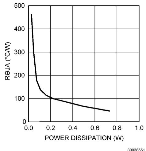
FIGURE 12. R<sub>θJA</sub> vs Internal Dissipation
