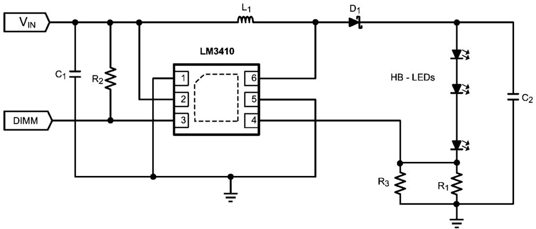
LM3410X (1.6MHz):  $V_{IN} = 2.7V$  to  $5.5V$ , 3 x  $3.4V$  LEDs, ( $V_{OUT} \approx 11V$ )  $I_{LED} \approx 340mA$
