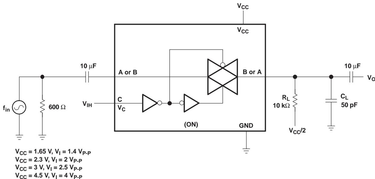
Figure 9. Sine-Wave Distortion
