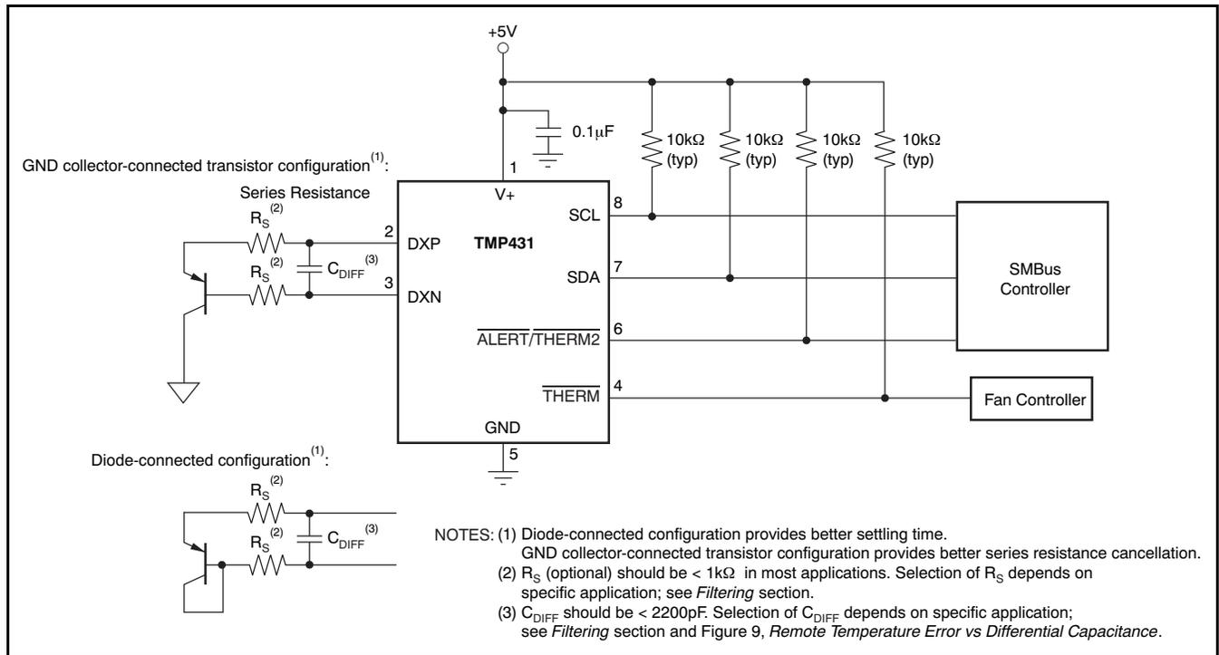
Figure 15. TMP431 Basic Connections
