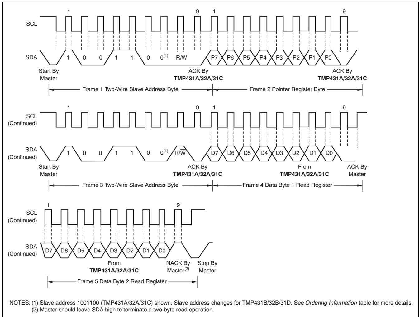
Figure 21. Two-Wire Timing Diagram for Two-Byte Read Format
