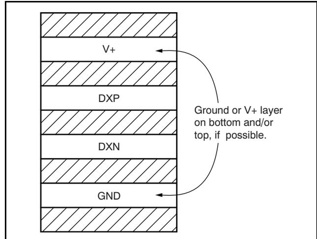
Note: Use 5 mil (.005 in, or 0,127 mm) traces with 5 mil (.005 in, or 0,127 mm) spacing.
