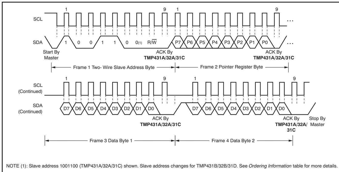
Figure 19. Two-Wire Timing Diagram for Write Word Format
