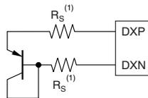
(1)  $R_S$  should be less than 1k $\Omega$ ; see [Filtering](#) section.
