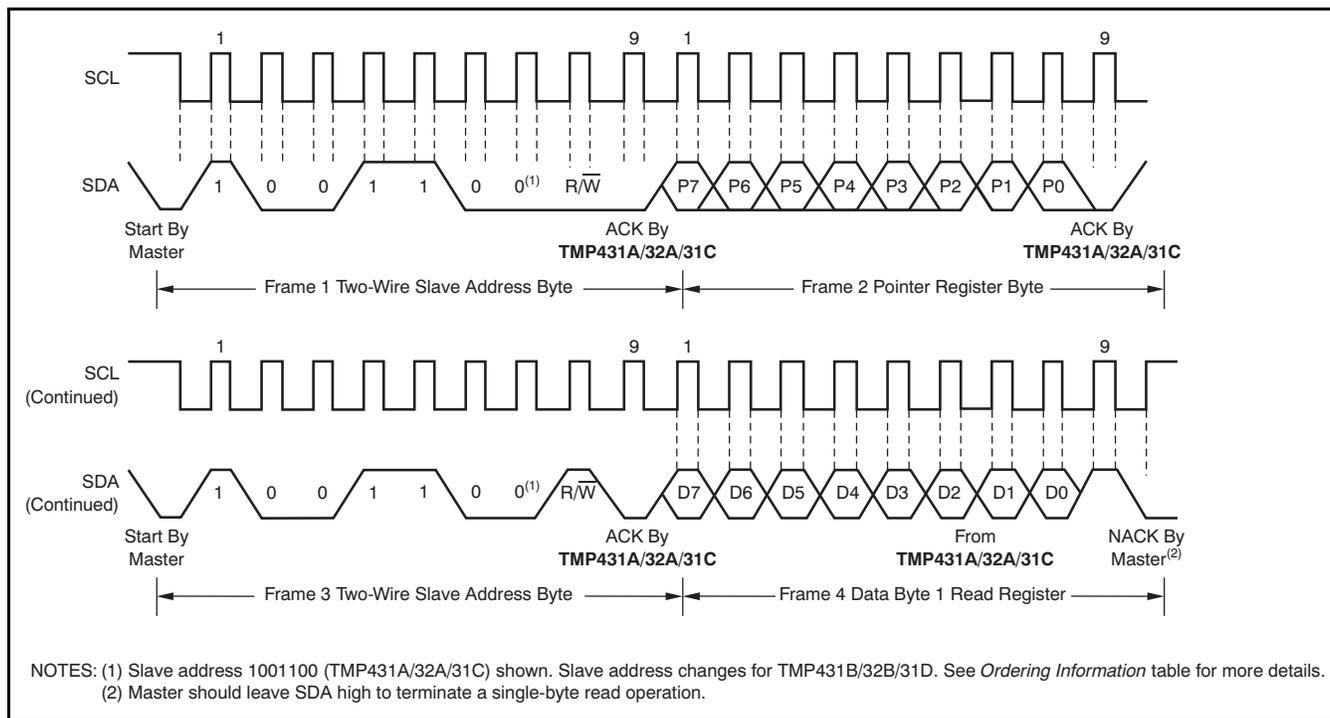
Figure 20. Two-Wire Timing Diagram for Single-Byte Read Format
