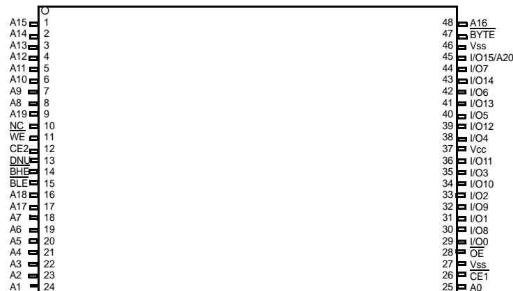
48-Pin TSOP-I (Forward)(1 M x 16 / 2M x 8) [5] Top View
