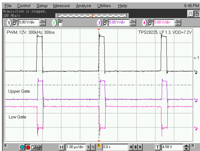
Figure 22. 12-V PWM Pulse at V_{DD} = 7.2 V
