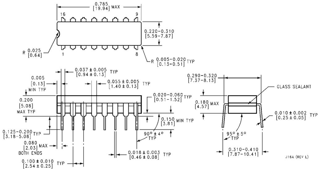
**16-Lead Ceramic Dual-in-Line Package**
