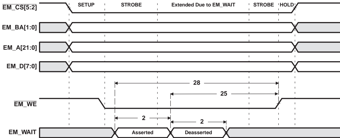
Figure 6-17. EM_WAIT Write Timing Requirements
