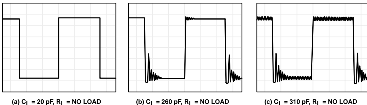
Figure 112. Effect of Capacitive Loads in Low-Bias Mode
