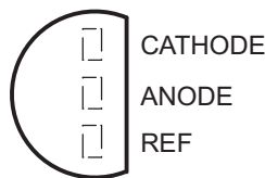
TLVH431 LP (TO-92/TO-226) PACKAGE (TOP VIEW)
