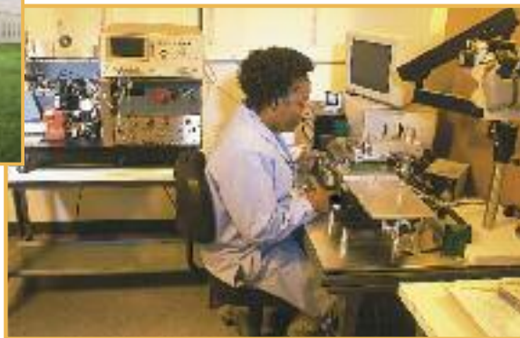
▶ Autopacking center packages chips into waffle packs
