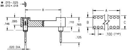
Description: DIP Dual In Line Socket Standard Solder Tail Open Frame Through Hole Plating Code: 93
