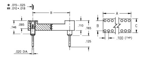
Open Frame Through Hole Plating Code: 99 Shell Plating: 200 μ" Tin/Lead(93/7) over 100 μ" Nickel Inner Contact Plating:
