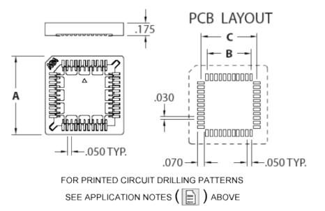
Description: PLCC Surface Mount PLCC Socket Standard Surface Mount Plating Code: 44 Shell Plating: 200  $\mu$ " Tin (matte finish) over 100  $\mu$ " Nickel Inner Contact Plating: 100  $\mu$ " Tin (matte finish) over 50  $\mu$ " Nickel Packaging: Packaged in Tubes
