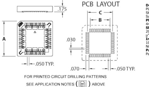
Description: PLCC Surface Mount PLCC Socket Standard Surface Mount Plating Code: 44 Shell Plating: 200  $\mu$ " Tin (matte finish) over 100  $\mu$ " Nickel Inner Contact Plating: 100  $\mu$ " Tin (matte finish) over 50  $\mu$ " Nickel Packaging: Packaged in Tubes
