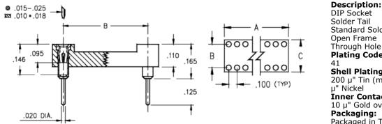
Standard Solder Tail (0.125 Tail) Open Frame Through Hole Plating Code: Shell Plating: 200 µ" Tin (matte finish) over 100 Inner Contact Plating: 10 µ" Gold over 50 µ" Nickel
