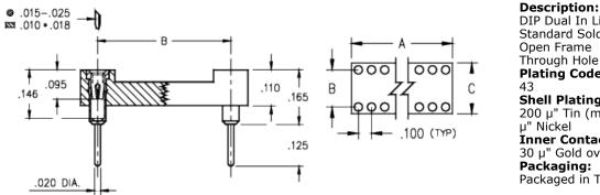
DIP Dual In Line Socket Standard Solder Tail Open Frame Through Hole Plating Code:
