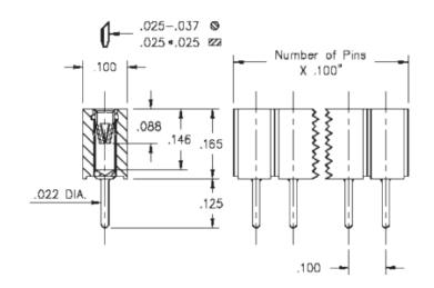
**Description:** Interconnect Socket Standard Solder Tail Socket Accepts .025" - .037" (0,635 - 0,94 mm)dia leads Single Row Through Hole
