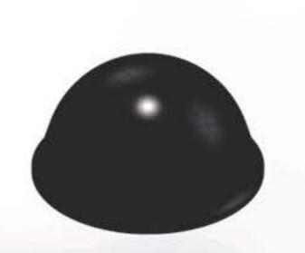
3M™ Bumpon™Protective Product SJ5017 is a self-adhesive rubber bumper designed to be used as feet, stops and spacers. The hemispherical shape provides excellent sound damping and energy absorption. Black, 0.750 in. wide x .380 in. high.
