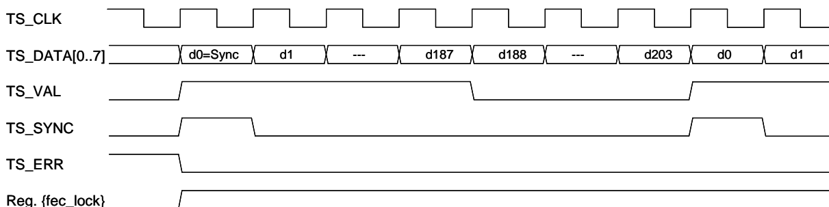
Figure 11. Continuous TS Parallel Mode with Rising Active Clock Edge and Enabled Parity Bytes
