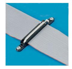
Secures stacked cables folds and breakouts plus laminated and molded bus bars. Mounting Application: Use one (1) base, one (1) corresponding size plate, and one (1) Intermediate cross section cable tie.
