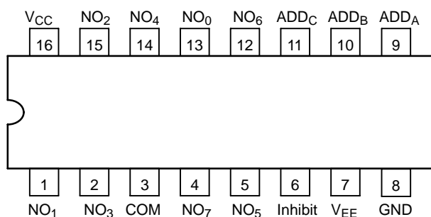
Figure 1. Pin Connection (Top View)
