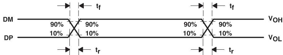
Figure 2. Differential Driver Timing Waveforms
