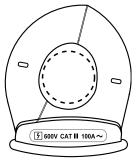
Jaw Opening: 1.10" (28mm) Conductor Size: 1" (26mm)
