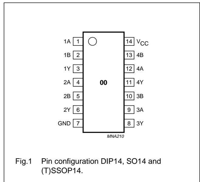
Fig.1 Pin configuration DIP14, SO14 and (T)SSOP14.
