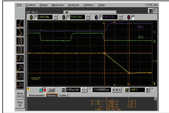
**FIGURE 2-99:** Half-Scale Settling Time (C00h to 400h) (MCP4726).
