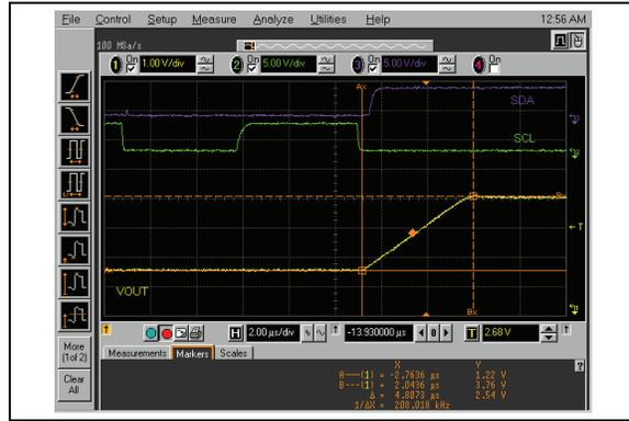
**FIGURE 2-98:** Half-Scale Settling Time (400h to C00h) (MCP4726).
