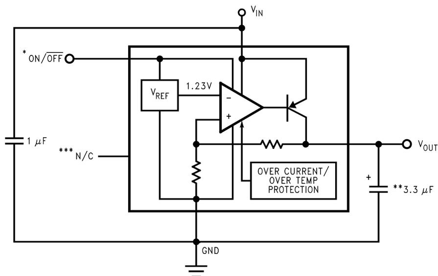
\*ON/OFF input must be actively terminated. Tie to  $V_{IN}$  if this function is not to be used.
