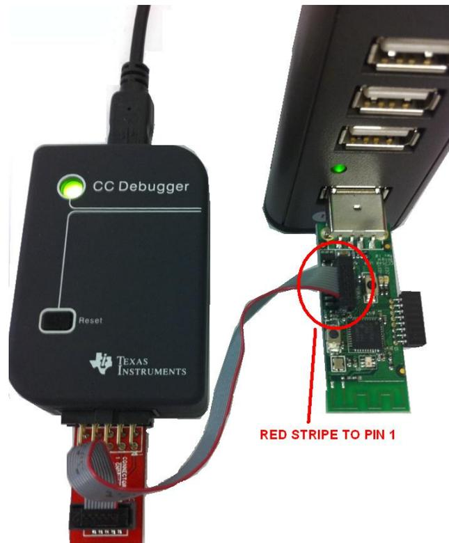
**Figure 11 CC2540 USB Dongle Connected to CC Debugger**
