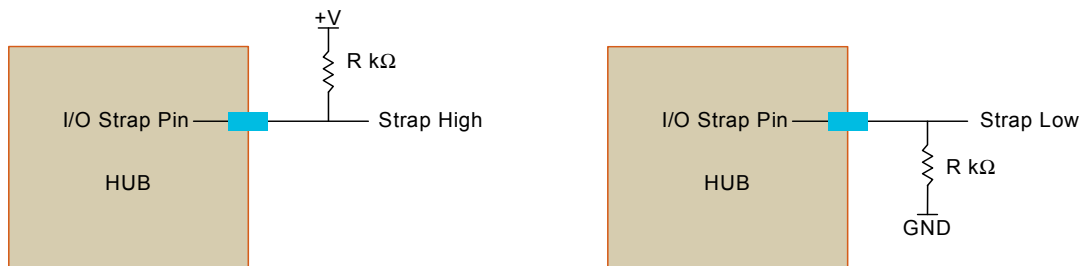
Figure 2.2 Non-Removable Pin Strap Example
