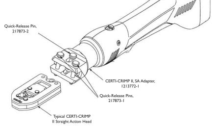
CERTI-CRIMP DA Battery Powered Crimp Tool Kit, Heads not included Part No. 1213804-( ) 110 V (-1 includes Ram Retract Switch; -3 without)
