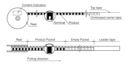
Reel Size : ¢178 Q'ty : 2000 pcs./Reel Packaging : Embossed Carrier Taping
