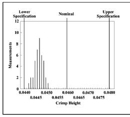
Figure 9-26 **CRIMP HEIGHT OFF TARGET**
