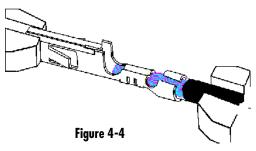
Pull force testing is a quick, destructive way to evaluate the mechanical properties of a crimp termination. When making a crimp, enough pressure must be applied to break down the oxides
