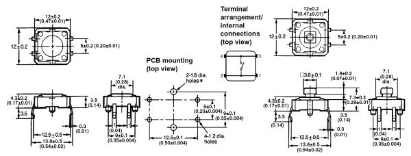
\* Fit the projection of the switch into this hole to secure the switch.
