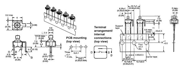
**Note:** Unless otherwise specified, a tolerance of  $\pm$  0.4 mm applies to all dimensions.
