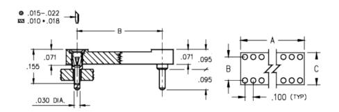
**Description:** DIP Socket Solder Tail Ultra Low Profile (0.095 Tail) Open Frame Through Hole Plating Code: 93 Shell Plating: 200 μ" Tin/Lead(93/7) over 100 μ" Nickel Inner Contact Plating:
