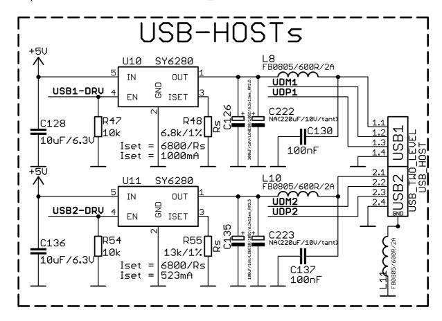
The USB\_HOST connector features two levels – called USB1 and USB2 in the schematic. The connector is situated between the USB\_OTG and the HDMI connector. Each of slots them features a low loss power distribution switch SY6280 which protects the board in case the devices you have plugged to each level USB\_HOST try to draw more than the allowed current.
