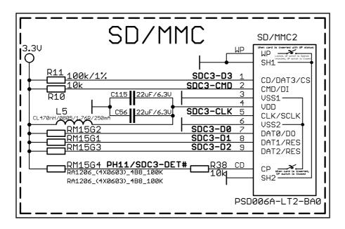
The SD/MMC2 slot is located on the back of the PCB and works with the "larger" SD and MMC cards. The connector was mounted to to popular demand.
